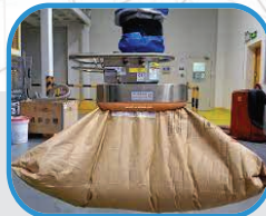
Vacuum Based Bag Lifting Mechanism – Nestlé
